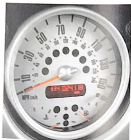
Figure 1.6 The speedometer of a vehicle that shows speeds in both miles per hour and kilometers per hour.
